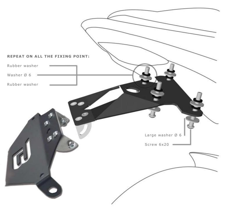
REMOVE THE ORIGINALE LICENCE PLATE FROM THE MOTORBIKE. APPLY BARRACUDA SPECIFIC BRACKET USING THE SCREWS IN THE KIT. FOLLOW THE PICTURE TO INSTALL AND FIX ALL. FINALLY APPROACH THE "X" LICENCE PLATE TO THE BRACKET FIXING IT WITH THE SPECIFIC SCREW.
