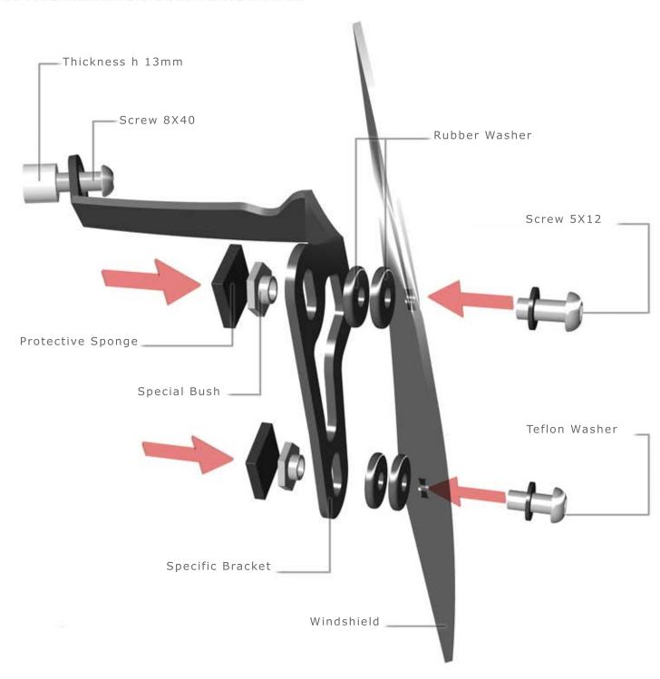
ASSEMBLE THE BARRACUDA WINDSHIELD/SCREEN USING THE SCREWS AND THICKNESS INCLUDED IN THE KIT. MOUNT ALL LIKE INSTRUCTION AND AT THE END UNSCREW THE SUPERIOR FORK SCREWS AND SUBSTITUE THEM WITH THE 8X40 SCREW TOGHETER THE THICKNESS H 13 WITH. WE ADVICE TO LOCK ALL ONCE YOU MOUNT THE WINDSHIELD/SCREEN TO AVOID PLEXIGLASS DAM-AGES DUE THE FORCING.
