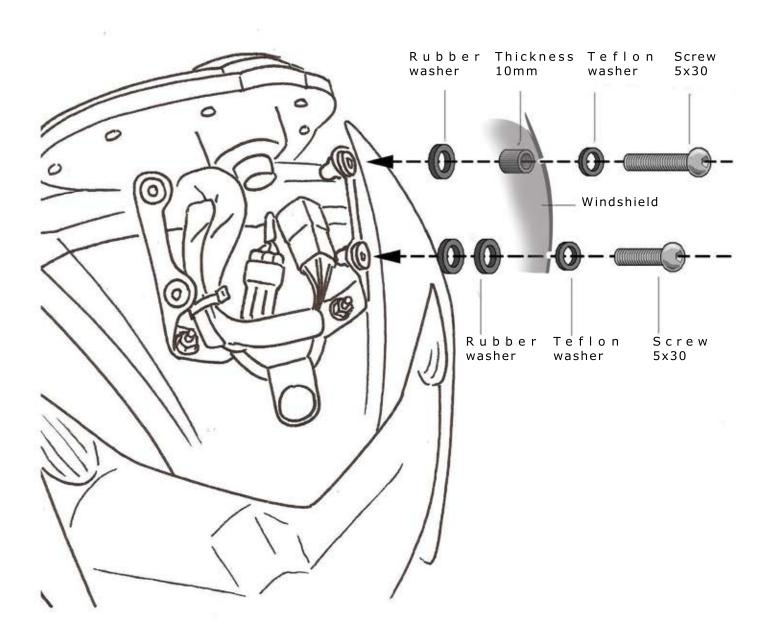
REMOVE THE ORIGINAL WINDSHIELD/SCREEN AND INSTALL THE BARRACUDA ONE FOLLOWING THE DESCRIPTION IN THE PICTURE: MOUNT THE TEFLON WASHERS BETWEEN THE HEAD OF SCREWS AND THE WINDSHIELD. LOCK THE SCREWS AFTER THE MOUNTING.
