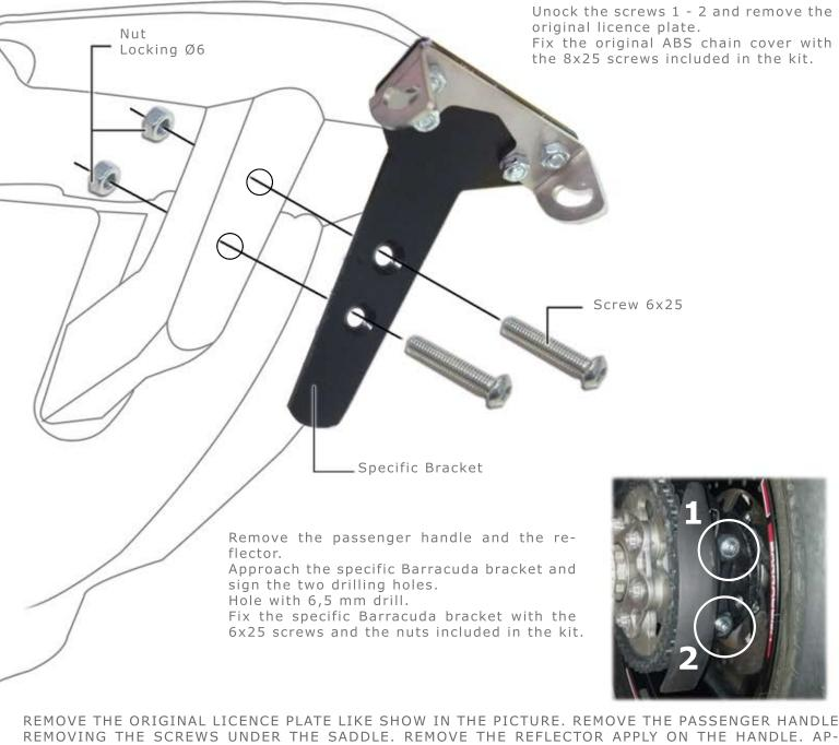
REMOVING THE SCREWS UNDER THE SADDLE. REMOVE THE REFLECTOR APPLY ON THE HANDLE. AP-PROACH THE SPECIFIC BARRACUDA BRACKET TO THE HANDLE LIKE SHOW IN THE PICTURE, FIND THE RIGHT POSITION, SIGN THE HOLES. PROCEED TO HOLE THE HANDLE WITH A 6,5 MM DRILL AND MOUNT AGAIN THE PASSENGER HANDLE. APPROACH THE "X" LICENCE PLATE TO THE BRACKET. THIS MODIFICATIONS DON'T CHANGE THE STRUCTURAL PARTS AND DON'T COMPROMISE THE MOTOR-BIKE SAFETY.
